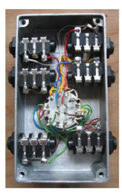
The ground of channel A (A -) is also the ground of the unit and is white. The signals of the channel A input (A in) and output (A out) are red. The ground of channel B (B -) is yellow. The signals of the channel B input (B in) and output (B out) are blue. The ground of the loop (L -) is brown. The signals of the loop output (L out) and input (L in) are blue.
