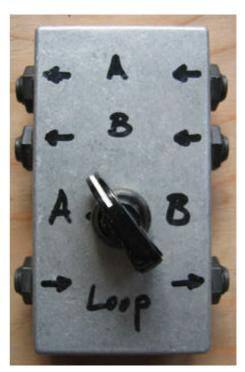
I found easily a 16 terminals 4P3T rotary switch, but was not able to find a toogle, rocker, or slide switch. Rocker and slide are not that easy to mount anyway.
